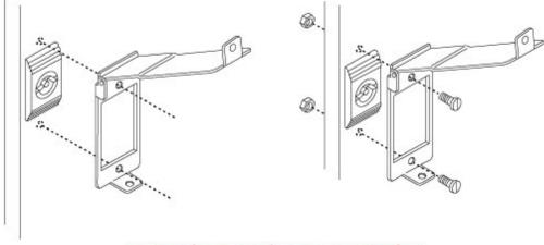
**Padlocking Lock System Installation**
