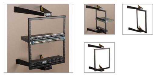
Open frame rack stores 12U of 19-inch rack equipment up to 18 inches deep in locations with limited floor space where a locked enclosure is not required. Pivots to allow easy rear access to equipment and cabling.
