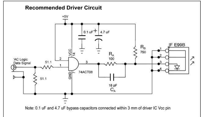
FIGURE 3. Typical interface circuit. (If = 35mA).
