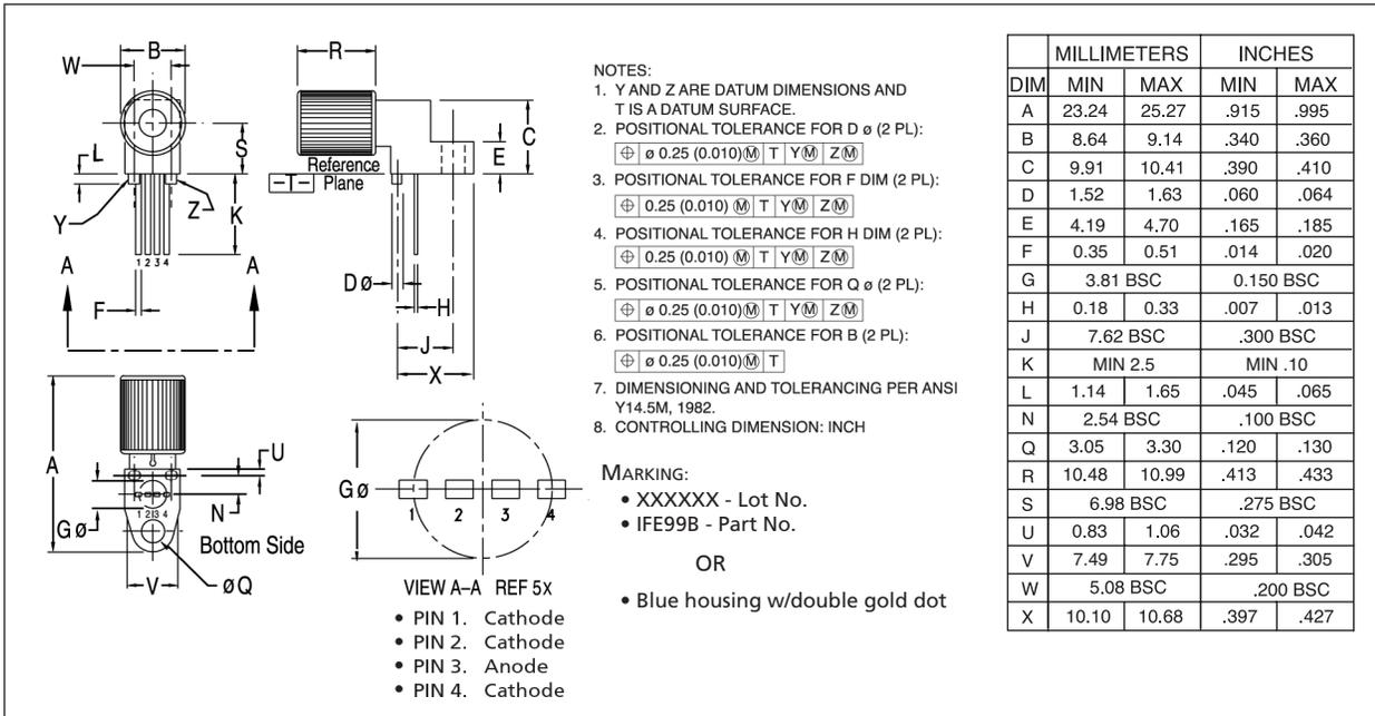
**FIGURE 6.** Case outline. Specifications are believed to be accurate but are subject to change. Industrial Fiber Optics assumes no responsibility for the consequences of using the information provided beyond replacement warranty for products not meeting stated specifications. Industrial Fiber Optics products are not authorized for use in life support applications without written approval from the President of Industrial Fiber Optics Corporation.
