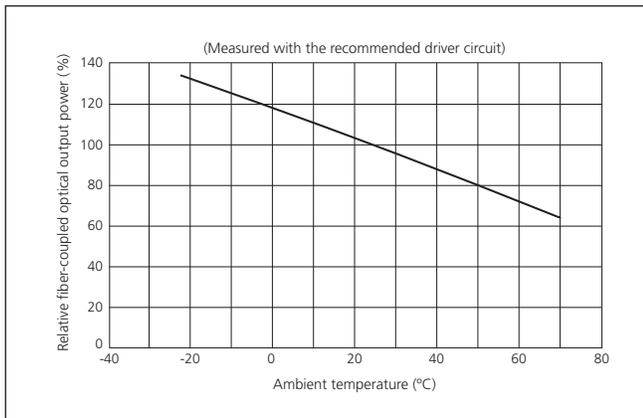
FIGURE 2. Optical power output versus temperature (If=20mA)
