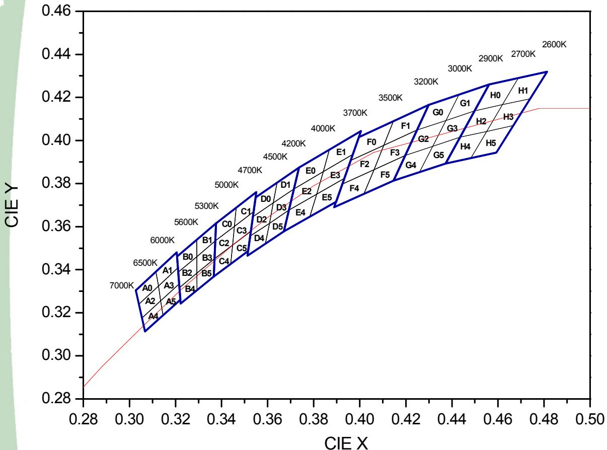
\* Apply the Energy Star binning(3200~7000K) & MACADAM 3 Step binning (just, 2600~3200K)
