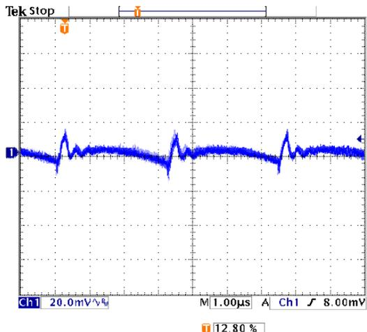
OKX2-T/16-D12-C On/Off Enable Startup Delay (V<sub>in</sub>=12V, V<sub>out</sub>=0.75V, I<sub>out</sub>=16A, C<sub>in</sub>=1000μF, C<sub>load</sub>=1μF // 10μF) Trace 1=Enable In, Trace 2=V<sub>out</sub>
