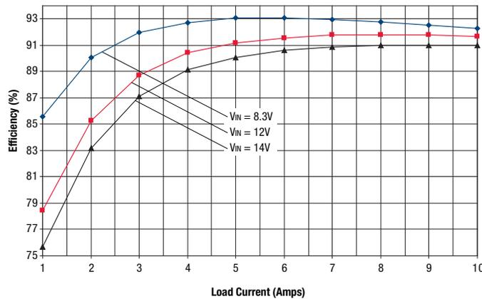
OKX2-T/10-D12 Efficiency vs. Line Voltage and Load Current @ +25°C
