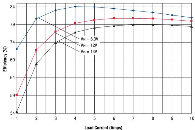
OKX2-T/10-D12 Efficiency vs. Line Voltage and Load Current @ +25°C
