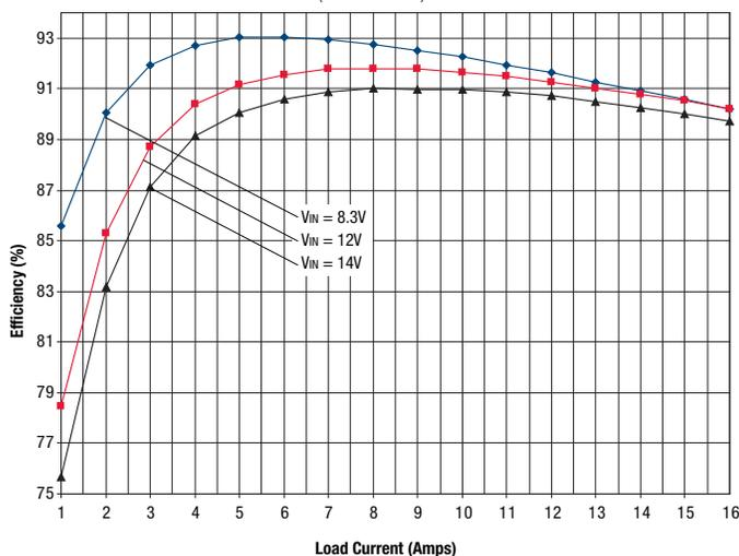
OKX2-T/16-D12 Efficiency vs. Line Voltage and Load Current @ +25°C
