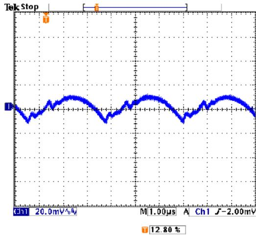
OKX2-T/16-D12-C Step Load Transient Response ( $V_{in}=12V$ ,  $V_{out}=3.3V$ ,  $C_{in}=1000\mu F$ ,  $C_{load}=0$ ,  $I_{out}=8A$  to  $16A$  to  $8A$ ) Trace1= $V_{out}$ , 200 mV/div., Trace4= $I_{out}$ , 5A/div.
