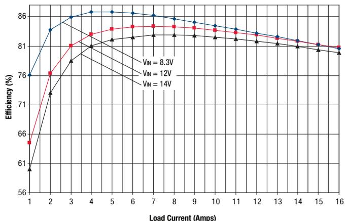
OKX2-T/16-D12 Efficiency vs. Line Voltage and Load Current @ +25°C
