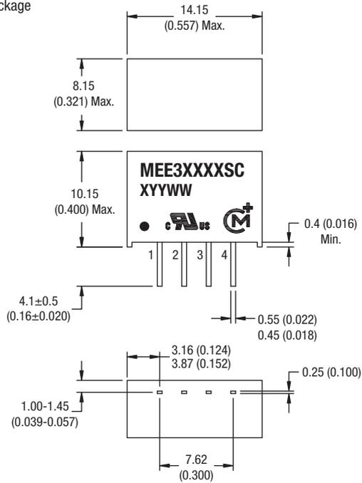
All dimensions in mm  $\pm 0.1$ mm (inches  $\pm 0.004$ ). All pins on a 2.54 (0.1) pitch and within  $\pm 0.25$  (0.01) of true position.
