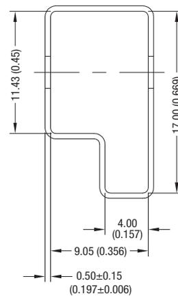
Unless otherwise stated all dimensions in mm (inches)  $\pm 0.5$ mm. Tube length: 520mm  $\pm 2$ mm (20.47).
