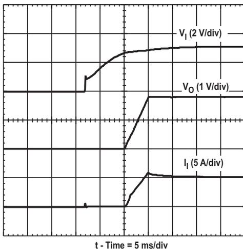
Figure 8. Power-Up Waveform
