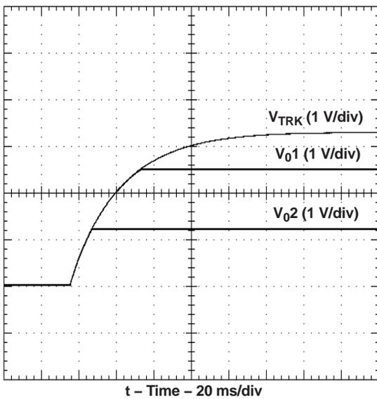
Figure 12. Simultaneous Power Up With Auto-Track Control
