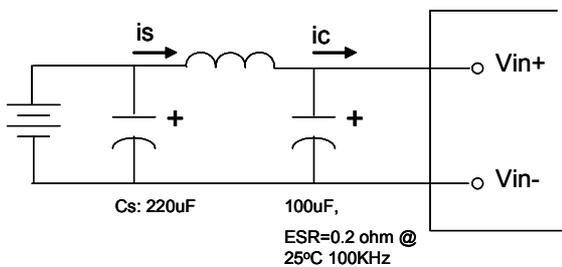
**Figure 11:** Test set-up diagram showing measurement points for Input Terminal Ripple Current and Input Reflected Ripple Current.
