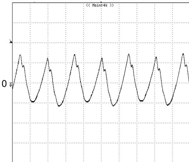
**Figure 15:** Output voltage ripple at nominal input voltage and rated full load current ( $20\text{ mV/div}$ ,  $2\mu\text{s/div}$ )
