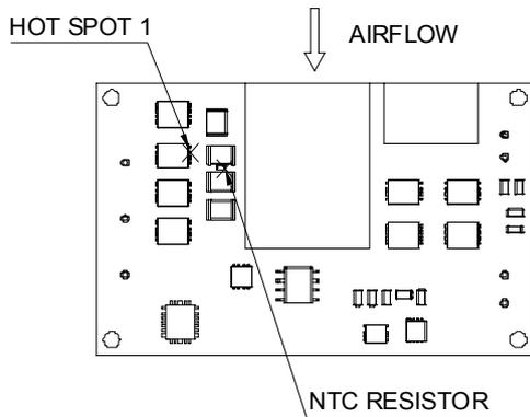
**Figure 18:** \* Hot spot 1 & NTC resistor temperature measured points
