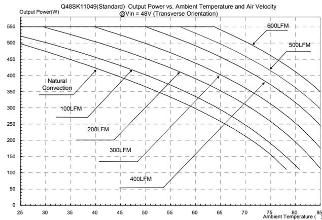
**Figure 19:** Output power vs. ambient temperature and air velocity @Vin=48V(Transverse Orientation, airflow from Vin+ to Vin-, without heat spreader)
