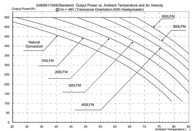
**Figure 21:** Output power vs. ambient temperature and air velocity @Vin=48V(Transverse Orientation, airflow from Vin+ to Vin-, with heat spreader)
