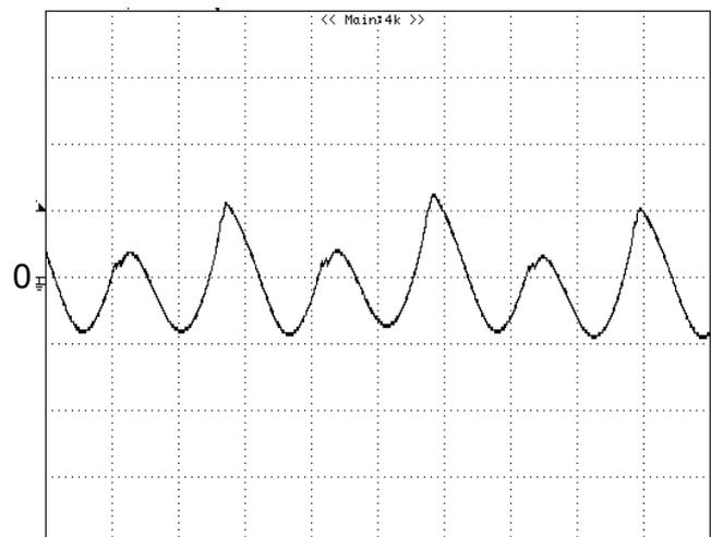
**Figure 12:** Input Terminal Ripple Current,  $i_c$ , at full rated output current and nominal input voltage with  $12\mu H$  source impedance and  $100\mu F$  electrolytic capacitor (100 mA/div, 2us/div).
