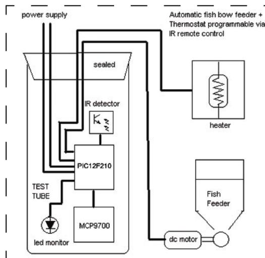
**Automatic Fish-Bowl Feeder and Thermostat:** Renato Kodaira's (Brazil) design uses a PIC12F210 and an MCP9700 to control the fish feeder and a electrical heater, with settings programmable via IR.
