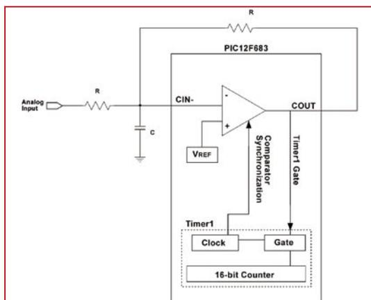
**Figure 2:** Delta-Sigma Converter Using the PIC12F683
