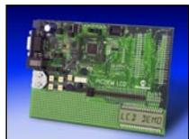
The **PICDEM™ LCD Development Board** (part # DM163028) demonstrates Microchip's family of microcontrollers with an integrated LCD driver module. Populated with the PIC18F8490 and designed for flexibility, this board supports additional LCD PIC® microcontrollers.
