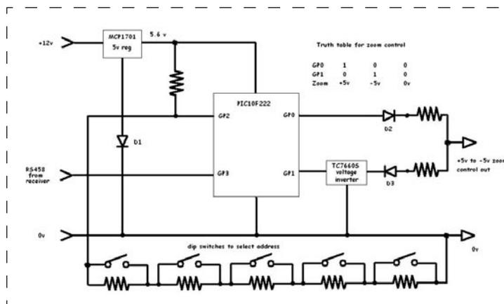
**You really CAN take the P&T out of PTZ:** submitted by Gordon Zerf (United Kingdom). This cost-effective remote control provides pan and tilt features to auto focus CCTV cameras using Microchip's PIC10F222, MCP1701 and TC76605 devices.
