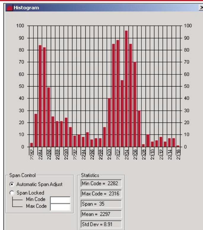
**Figure 1:** This histogram plot shows data from an ADC that is bimodal. It is difficult, if not impossible, to apply digital filtering to this data to recover a digital code that actually represents the input analog voltage accurately.
