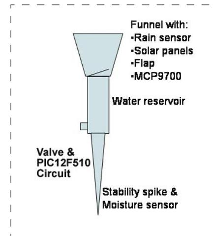
**The Rose Protector:** submitted by Maarten Hoffman (USA). This device protects roses by providing adequate water based on moisture and temperature using Microchip's PIC12F510 and MCP9700 devices.
