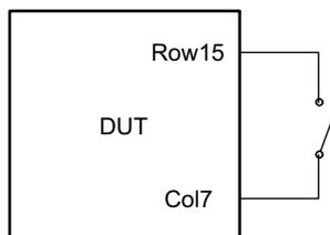
Figure 14. Row Pull-down Load Configuration
