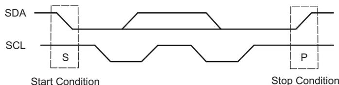
**Figure 1. Definition of Start and Stop Conditions**
