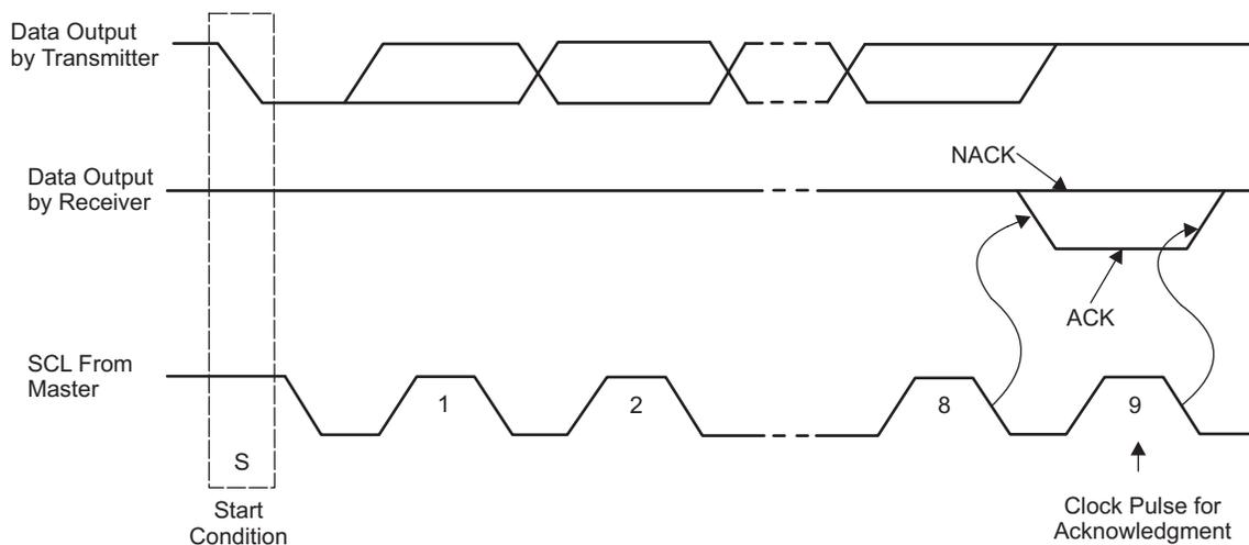
**Figure 3. Acknowledgment on I<sup>2</sup>C Bus**
