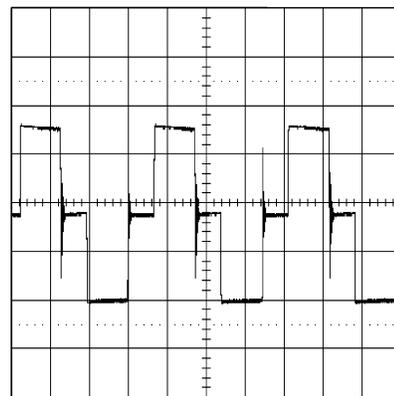
Conditions: Input Voltage = 36VDC Output Current = 10A Trace: Q2 drain to source voltage Volts/div = 10V Horizontal Resolution = 2  $\mu$ sec/div
