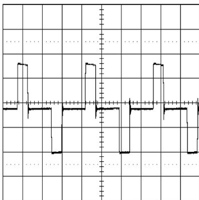
Conditions: Input Voltage = 72VDC Output Current = 10A Trace: Q2 drain voltage Volts/div = 20V Horizontal Resolution = 2  $\mu$ sec/div
