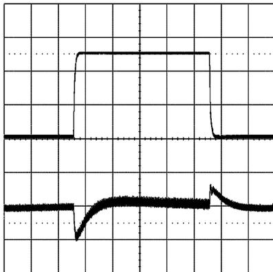
Conditions: Input Voltage = 48VDC Output Current = 5A to 10A Bandwidth Limit = 20 MHz Traces: Top Trace: Output Current Amps/div = 5A Bottom Trace: Output Voltage response Volts/div = 100 mV Horizontal Resolution = 200  $\mu$ sec/div
