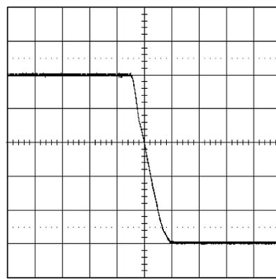
Conditions: Input Voltage = 48VDC Trace: Output Voltage Volts/div = 1V Horizontal Resolution = 1 msec/div
