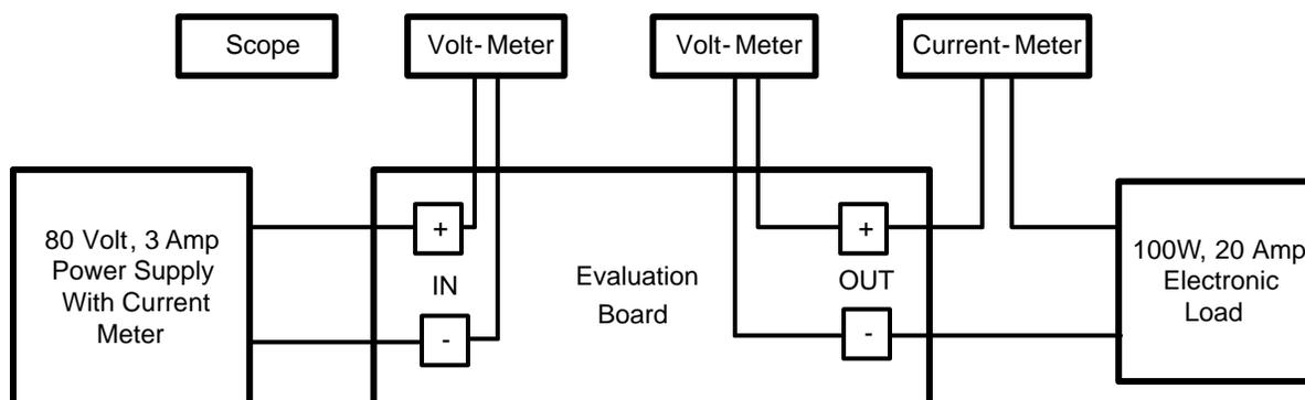
**Figure 2. Typical Application Set-up**
