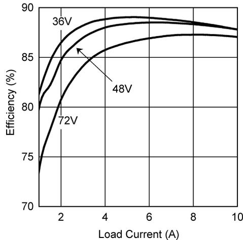
**Figure 3. Efficiency vs. Load Current and VIN**
