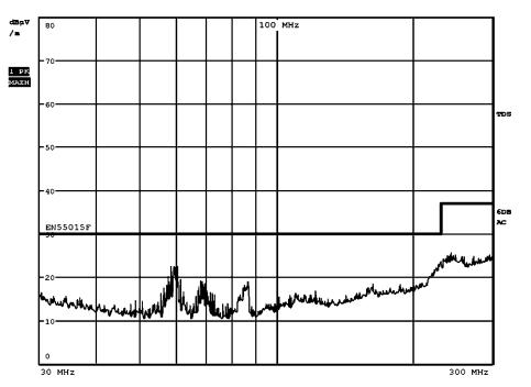
Figure 38. Complies with EN55015 Radiated Emissions (VERT. / HEIGHT=1.0m / RANGE=10m)  $C_{IN} = 2.2\mu$ F,  $C_{OUT} = 2.2\mu$ F,  $V_{IN} = 60$ V,  $I_{LED} = 350$ mA, No. of LED = 16
