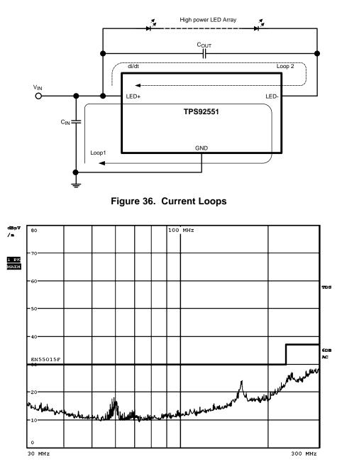
Figure 37. Complies with EN55015 Radiated Emissions (HORI. / HEIGHT=3.0m / RANGE=10m)  $C_{IN} = 2.2 \mu F$ ,  $C_{OUT} = 2.2 \mu F$ ,  $V_{IN} = 60 V$ ,  $I_{LED} = 350 mA$ , No. of LED = 16
