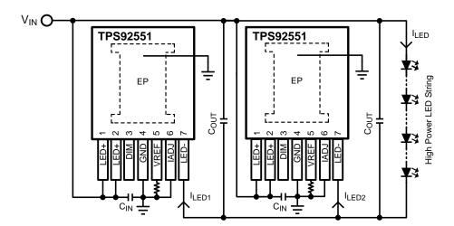
Figure 34. Parallel Operation Circuit Schematic for I<sub>LED</sub> = 900mA
