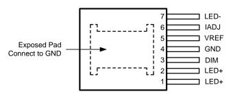
Figure 5. 7-Pin PFM (Top View) See NDW0007A Package
