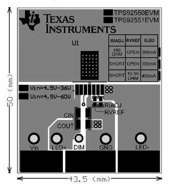
Figure 39. Top Layer and Top Overlay
