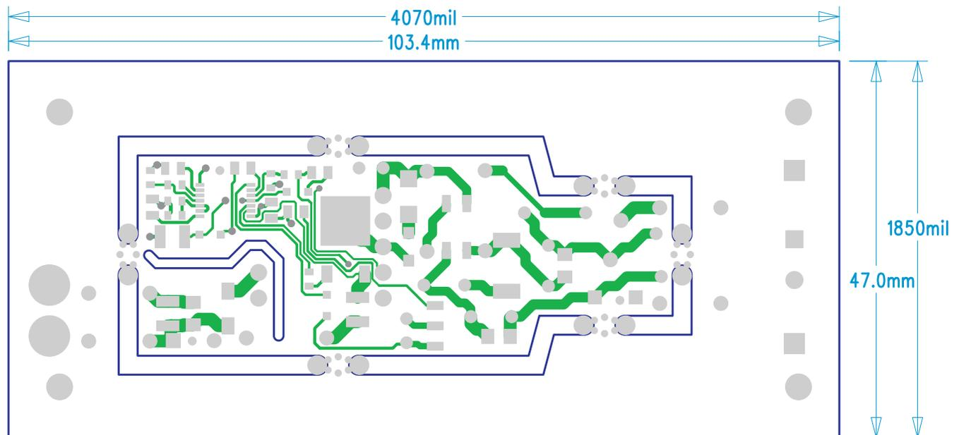
Figure 30. LM3447-A19-120VEVM Bottom Layer Copper (bottom view)
