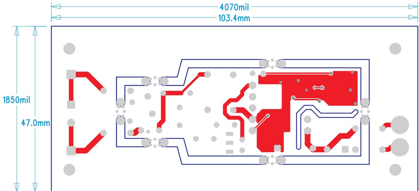
Figure 29. LM3447-A19-120VEVM Top Layer Copper (top view)
