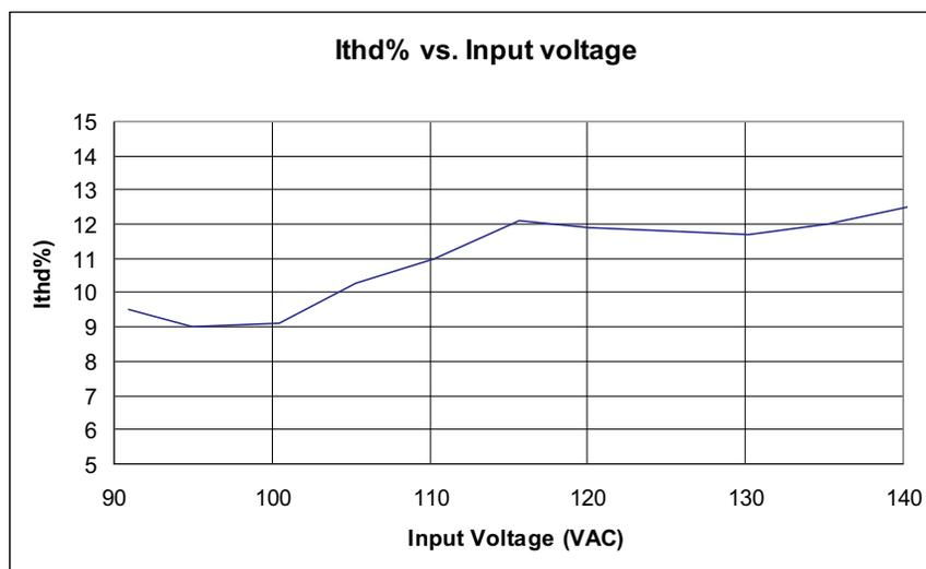
Figure 7. LM3447-A19-120VEVM- Ithd % vs Line Voltage
