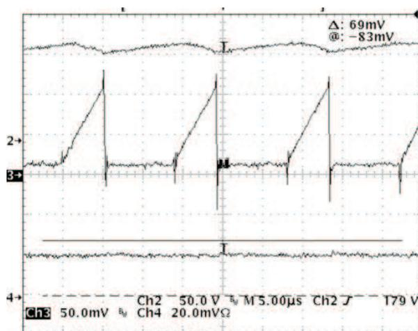
Figure 20. Current Sense Waveform
