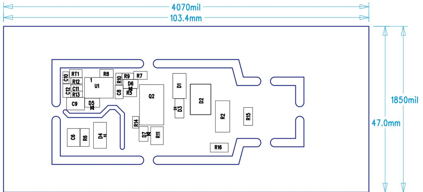
**Figure 32. LM3447-A19-120VEVM Bottom Assembly Drawing (bottom view)**
