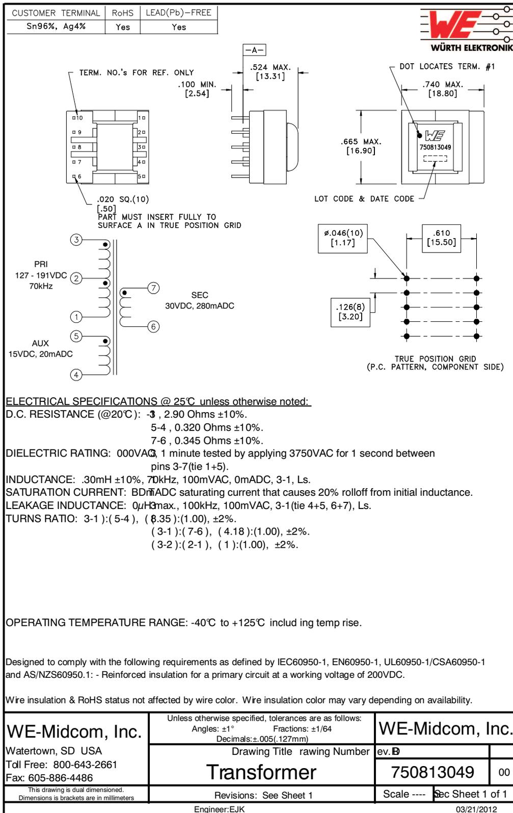
**Figure 28. Transformer Specification**
