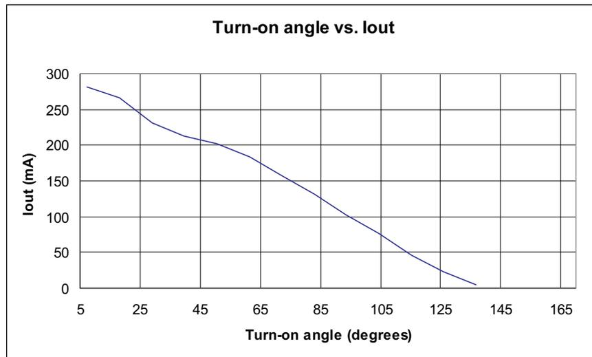
**Figure 10. LED Current vs Conduction Angle**
