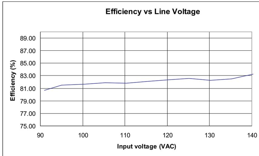
Figure 3. LM3447-A19-120VEVM Efficiency
