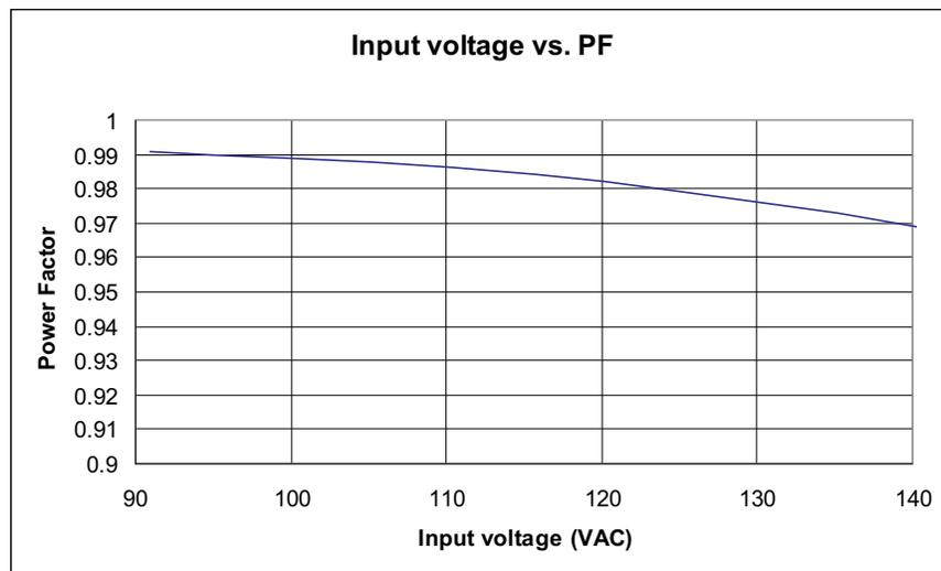
Figure 4. LM3447-A19-120VEVM Power Factor vs Line Voltage
