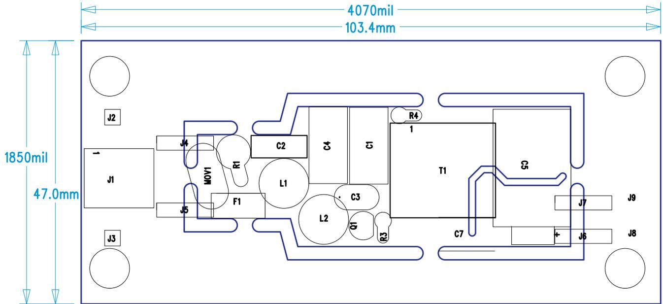
**Figure 31. LM3447-A19-120VEVM Top Assembly Drawing (top view)**
