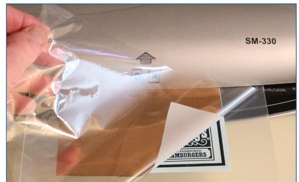
Shown with Carrier Board supporting printed page overlaid with foil, passing through the laminator.
