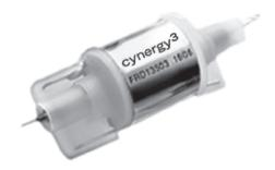
A complete RF screen around the coil assembly for a low loss transmission path, results in better carry current at elevated temperatures for this open frame series. An anti-corona sleeve is tted around the reed switch for improved RF voltage isolation. This type is widely used in HF Antenna Tuning Unit (ATU) applications.
