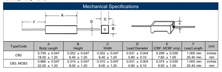
Ceramic Housed with Axial Leads Power Resistor
