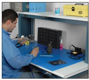
Figure 6. Using the Chargebuster Ion Gun
