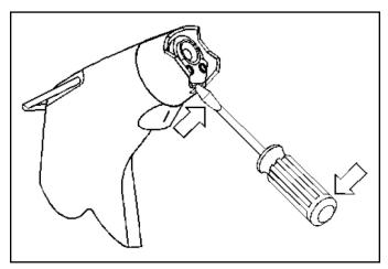
Figure 6. Inserting a screwdriver into the slot located at the bottom of the gun's nozzle
