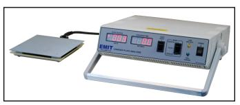
Figure 7. EMIT 50571 Charged Plate Analyzer
