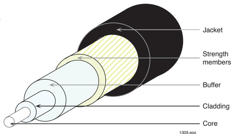
**Figure 3. Cross-section of a typical optical cable.**
