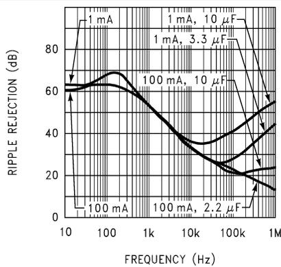
**Figure 5-41. Ripple Rejection versus Frequency (Legacy Chip)**
