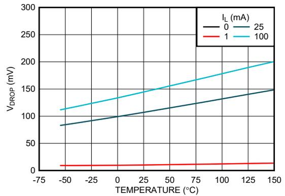
Figure 5-12. Dropout Voltage ( $V_{DO}$ ) versus Temperature (New Chip)
