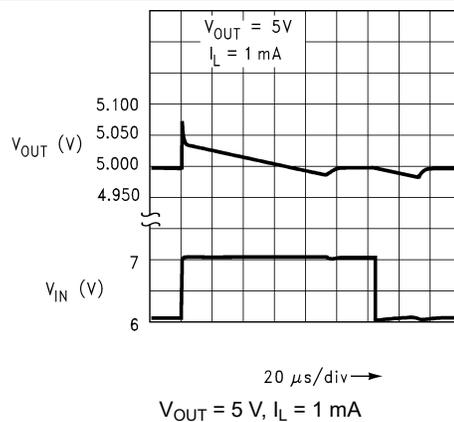
Figure 5-24. Line Transient Response (Legacy Chip)
