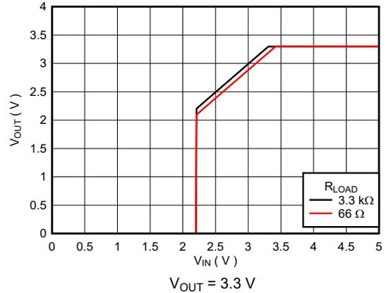
Figure 5-8. Output Voltage versus  $V_{IN}$  (New Chip)
