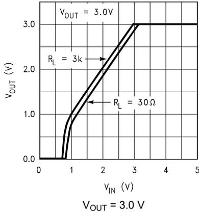
Figure 5-7. Output Voltage versus  $V_{IN}$  (Legacy Chip)
