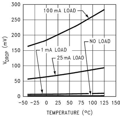
Figure 5-11. Dropout Voltage ( $V_{DO}$ ) versus Temperature (Legacy Chip)
