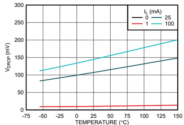
Dropout Voltage versus Temperature (New Chip)
