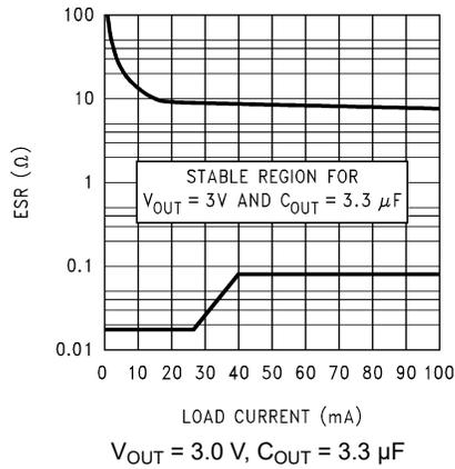
Figure 7-5. 3.0-V, 3.3- $\mu\text{F}$  ESR Curves (Legacy Chip)
