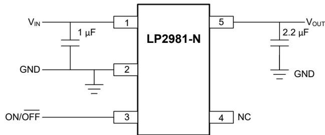
\*ON/  $\overline{\text{OFF}}$  input must be actively terminated. Tie to  $V_{\text{IN}}$  if this function is not to be used. Minimum output capacitance is shown to insure stability over full load current range. More capacitance provides superior dynamic performance and additional stability margin (see [Section 7.1.1](#)).
