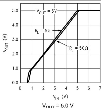
**Figure 5-5. Output Voltage versus  $V_{IN}$  (Legacy Chip)**
