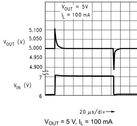
Figure 5-22. Line Transient Response (Legacy Chip)
