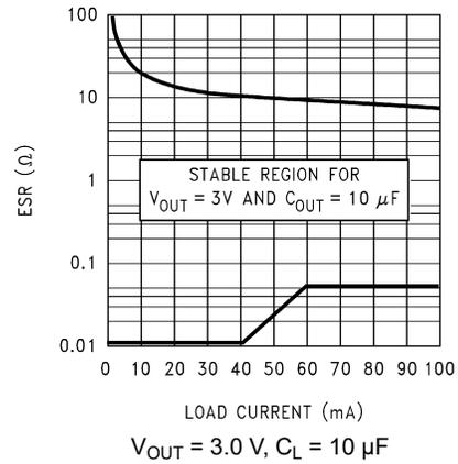
Figure 7-6. 3.0-V, 10- $\mu\text{F}$  ESR Curves (Legacy Chip)
