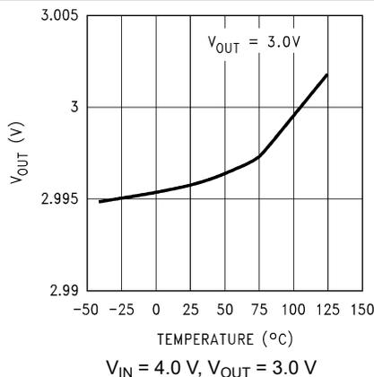
**Figure 5-3. Output Voltage versus Temperature (Legacy Chip)**
