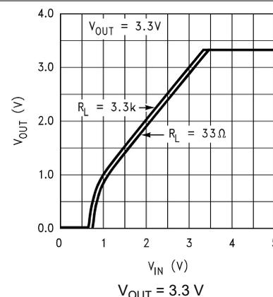
**Figure 5-6. Output Voltage versus  $V_{IN}$  (Legacy Chip)**
