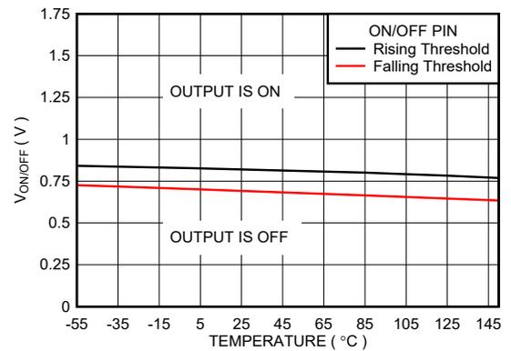
Figure 5-58. ON/  $\overline{\text{OFF}}$  Threshold versus Temperature (New Chip)
