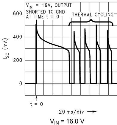
Figure 5-33. Short Circuit Current versus Time (Legacy Chip)
