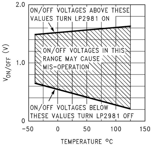
Figure 5-57. ON/  $\overline{\text{OFF}}$  Threshold versus Temperature (Legacy Chip)
