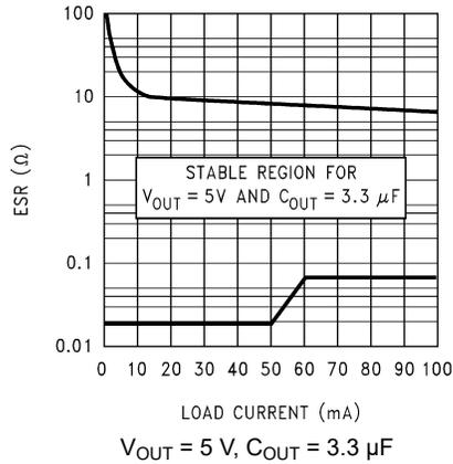
Figure 7-3. 5-V, 3.3- $\mu\text{F}$  ESR Curves (Legacy Chip)
