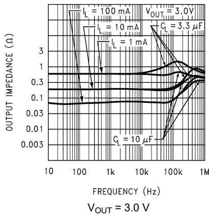
**Figure 5-39. Output Impedance versus Frequency (Legacy Chip)**
