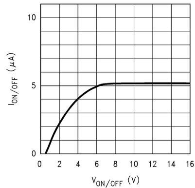
Figure 5-54. ON/OFF Pin Current versus  $V_{ON/OFF}$  (Legacy Chip)
