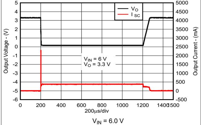
Figure 5-32. Short Circuit Current versus Time (New Chip)
