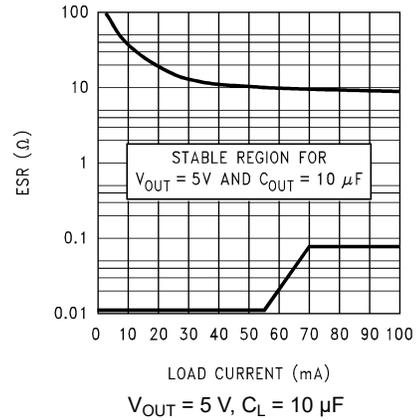
Figure 7-4. 5-V, 10- $\mu\text{F}$  ESR Curves (Legacy Chip)
