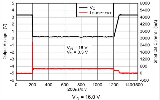
Figure 5-34. Short Circuit Current versus Time (New Chip)
