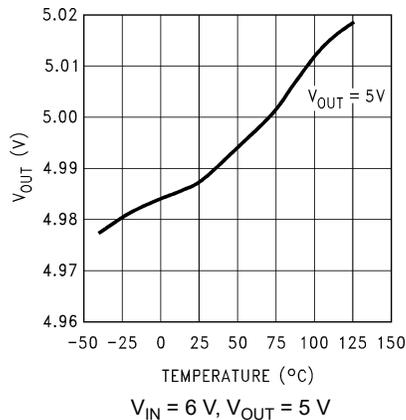
**Figure 5-1. Output Voltage versus Temperature (Legacy Chip)**
