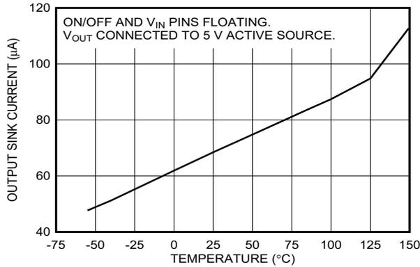
Figure 5-49. Output Reverse Leakage versus Temperature (New Chip)
