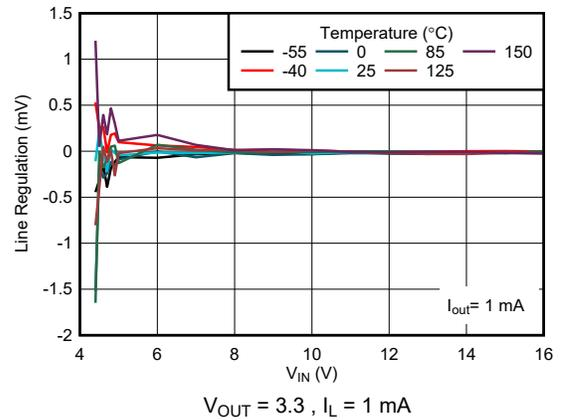
Figure 5-10. Line Regulation versus  $V_{IN}$  & Temperature (New Chip)
