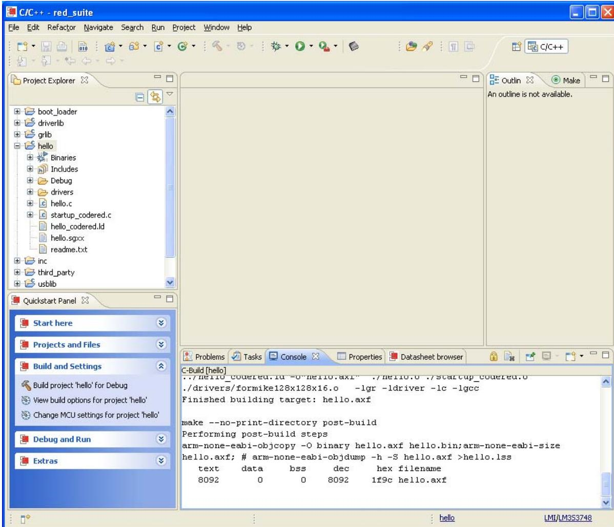
6. To rebuild an individual project, select the project you want to build by clicking an item in the Project Explorer list. From the “Build and Settings” section of the Quickstart Panel in the bottom left of the Red Suite window, click “Build project ‘<name>’ for Debug.” If this option is not visible, expand the “Build and Settings” section by clicking on the downward pointing arrows to the right of the title.
