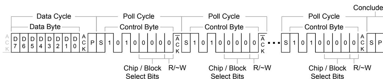
Figure 8.6 I<sup>2</sup>C EEPROM Byte Write
