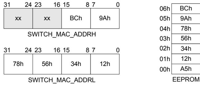
**Figure 13.2 Example SWITCH\_MAC\_ADDRL, SWITCH\_MAC\_ADDRH, and EEPROM Setup**
