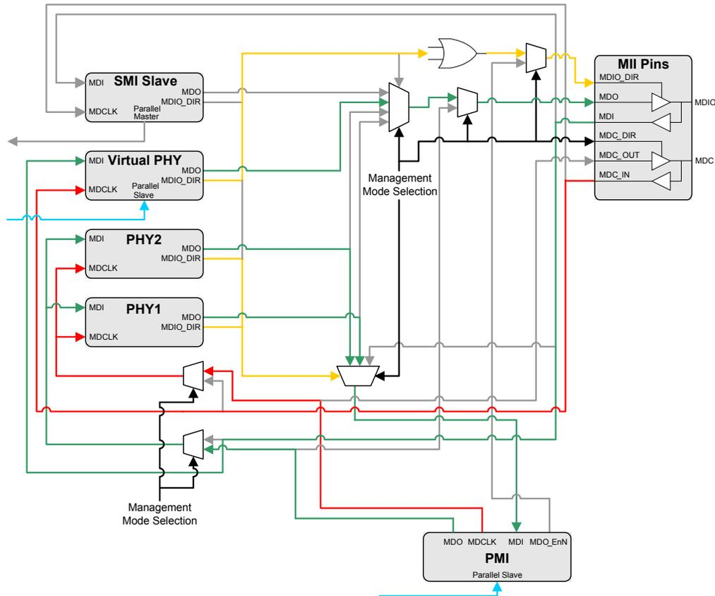
Figure 9.6 MII Mux Management Path Connections - PHY Mode I<sup>2</sup>C/SPI Managed
