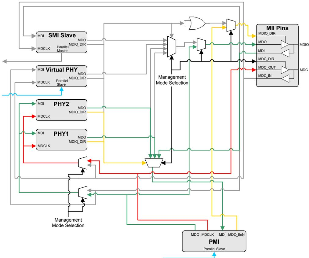
Figure 9.3 MII Mux Management Path Connections - MAC Mode I<sup>2</sup>C/SPI Managed
