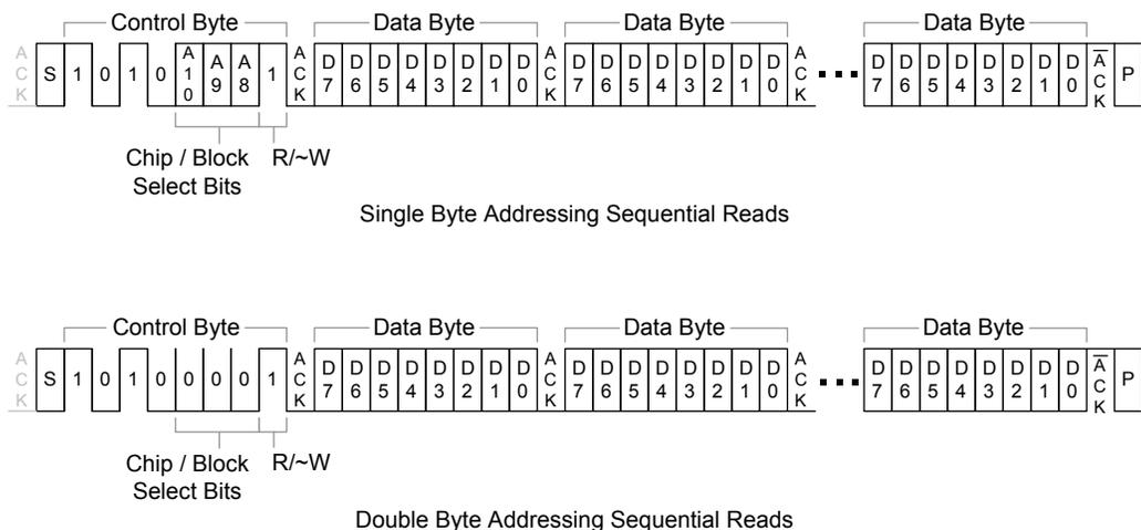
Figure 8.5 I<sup>2</sup>C EEPROM Sequential Byte Reads
