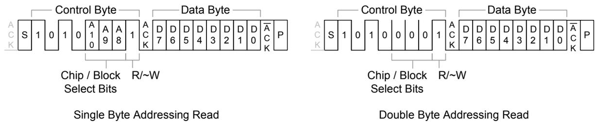
Figure 8.4 I<sup>2</sup>C EEPROM Byte Read
