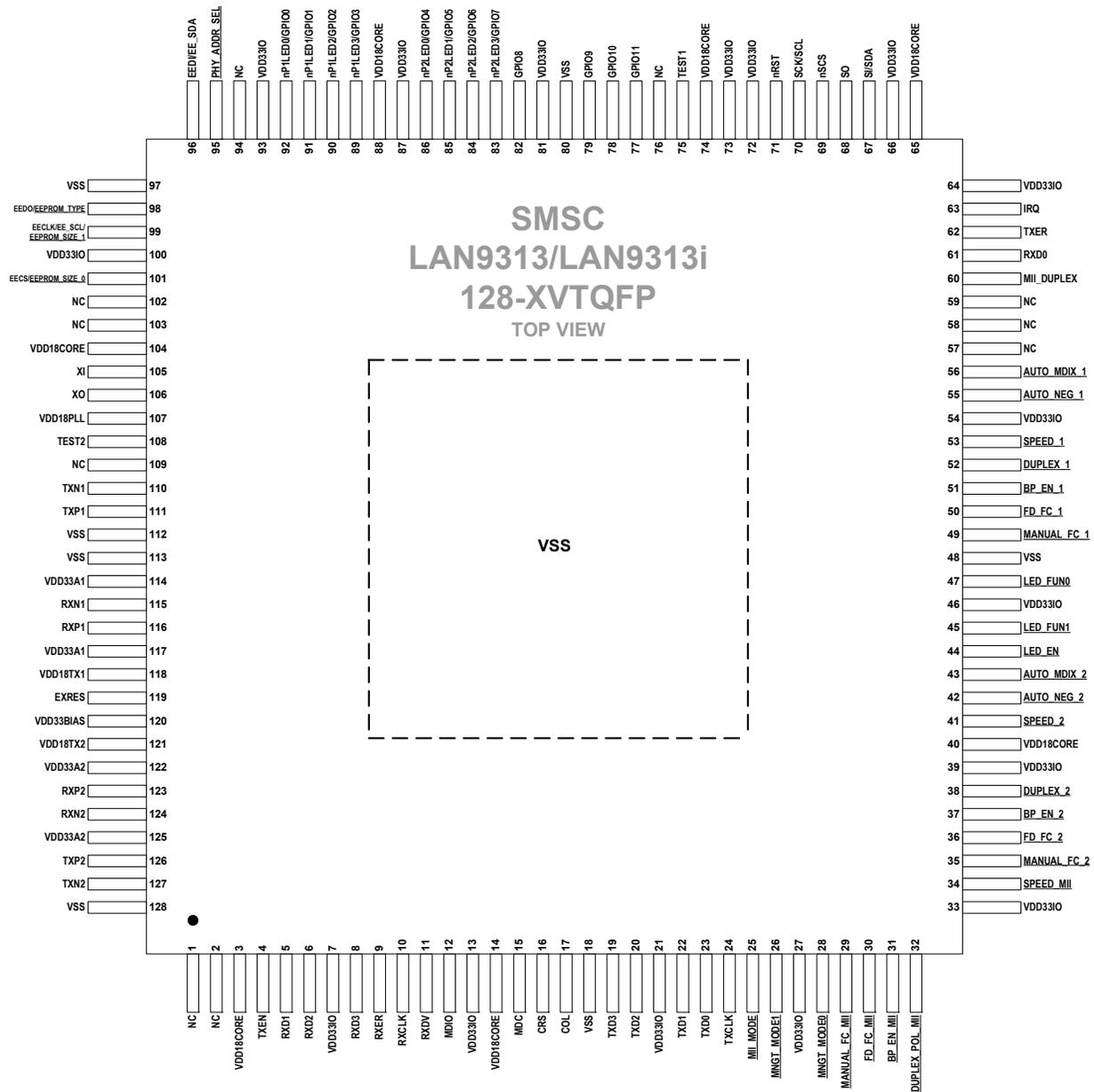
Figure 3.2 LAN9313/LAN9313i 128-XVTQFP Pin Assignments (TOP VIEW)
