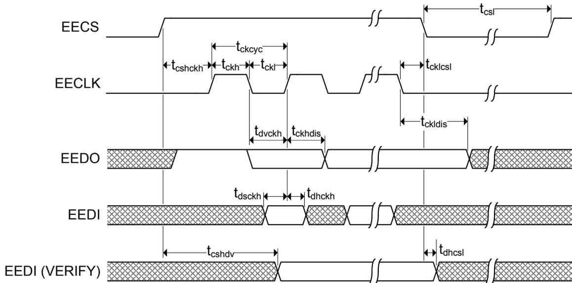
Figure 14.4 Microwire Timing
