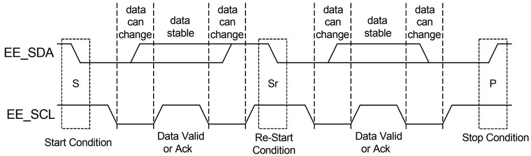
Figure 8.2 I<sup>2</sup>C Cycle
