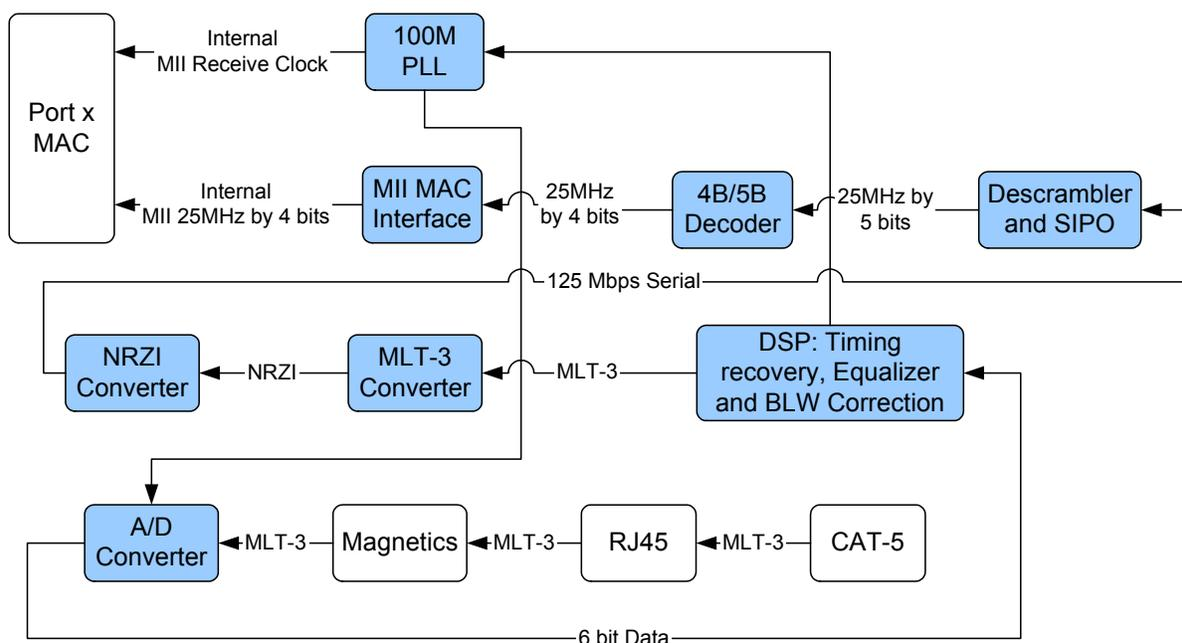
Figure 7.3 100BASE-TX Receive Data Path
