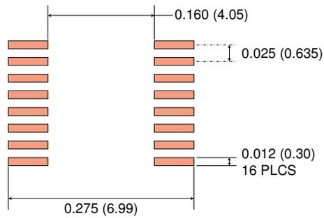
**0.15" Narrow-Body 16-pin SOIC Pad Layout**
