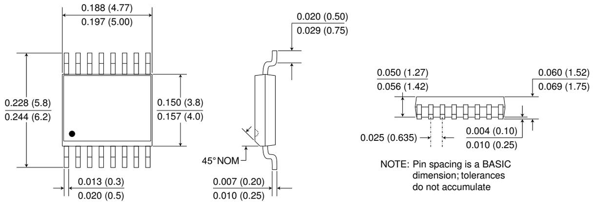
**0.15" 16-pin Narrow-Body SOIC Package (-3 suffix)**
