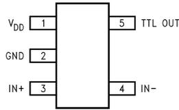
**Figure 3-1. Top View See Package Number DBV (R-PDSO-G5)**
