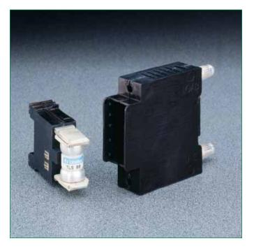
Littelfuse compact LTFD 101 fuseholders for TLS fuses are designed for quick installation into telecom equipment panels. Their modular design fits into spaces originally designed for circuit breakers and they can be front panel mounted or rear mounted using bullet connectors. The innovative new pull-out design eliminates the need for tools to replace fuses and includes an alarm signaling circuit to identify the blown fuse.
