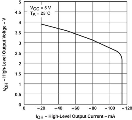
**Figure 5-1. High-level Output Voltage vs High-level Output Current**
