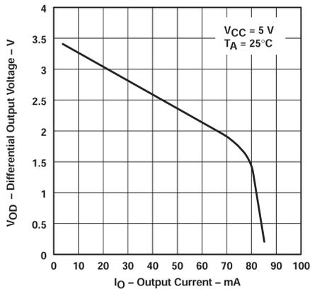
**Figure 5-3. Differential Output Voltage vs Output Current**
