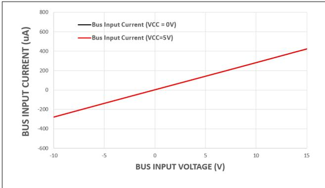
Figure 5-1. Bus Input Current vs Bus Input Voltage
