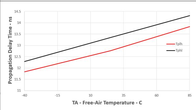
Figure 5-4. Propagation Delay Time vs Free-air Temperature
