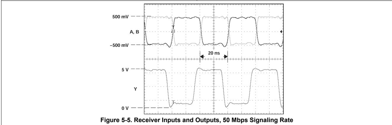
Figure 5-5. Receiver Inputs and Outputs, 50 Mbps Signaling Rate
