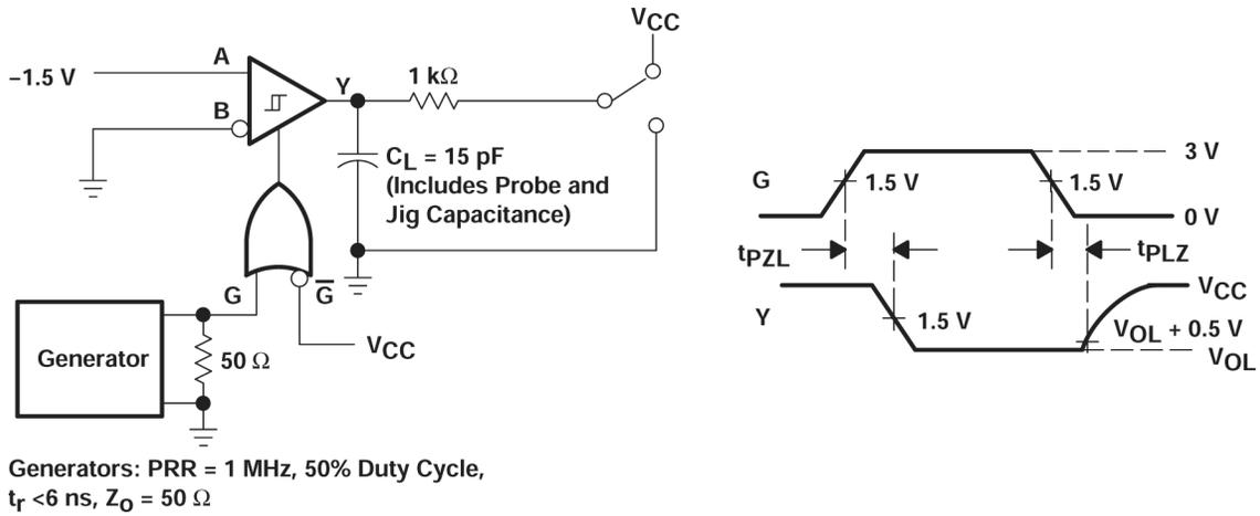
**Figure 6-4. Test Circuit Waveforms,  $t_{pZL}$  and  $t_{pLZ}$**
