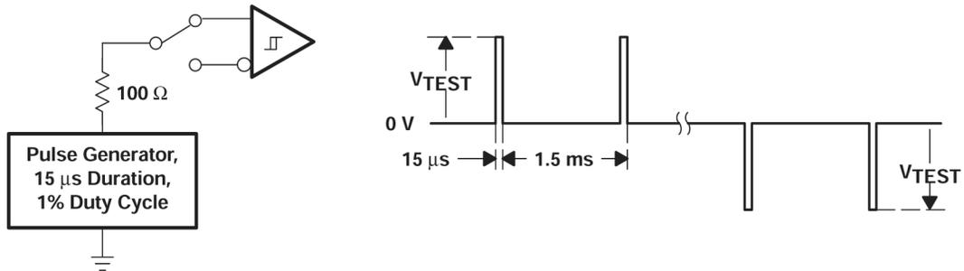
**Figure 6-5. Test Circuit and Waveform, Transient Over-Voltage Test**
