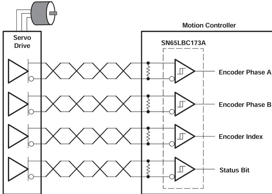
Figure 8-2. Typical Application Circuit, High-Speed Servomotor Encoder Interface
