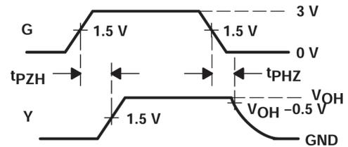
Figure 6-3. Test Circuit Waveforms,  $t_{PZH}$  and  $t_{PHZ}$
