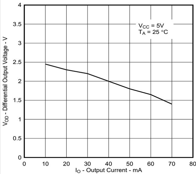
**Figure 6-3. Driver Differential Output Voltage vs Output Current**
