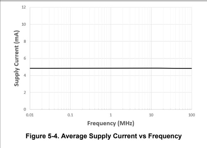
Figure 5-4. Average Supply Current vs Frequency
