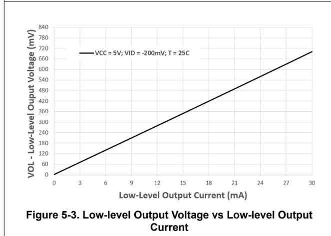
Figure 5-3. Low-level Output Voltage vs Low-level Output Current
