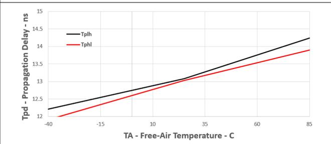
Figure 5-6. Propagation Delay Time vs Free-air Temperature
