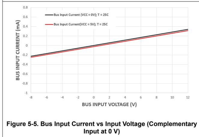
Figure 5-5. Bus Input Current vs Input Voltage (Complementary Input at 0 V)
