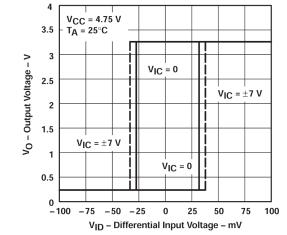
Figure 5-1. Output Voltage vs Differential Input Voltage
