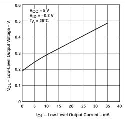
Figure 5-4. Low-level Output Voltage vs Low-level Output
