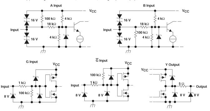
Figure 7-1. Equivalent Input and Output Schematic Diagrams
