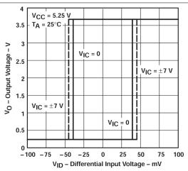
Figure 5-2. Output Voltage vs Differential Input Voltage
