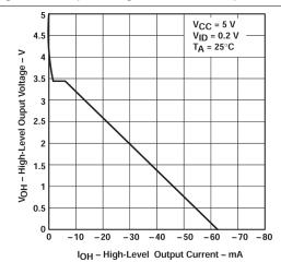
Figure 5-3. High-level Output Voltage vs High-level Output Current
