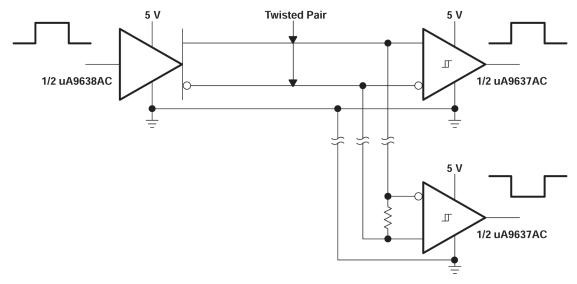
Figure 8-1. EIA/TIA-422-B System Applications
