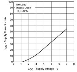
Figure 5-5. Supply Current vs Supply Voltage
