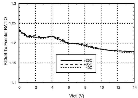
[1] Rejection ratio is defined as the ratio of the frequency at which the relative insertion loss is 20 dB to f<sub>center</sub>
