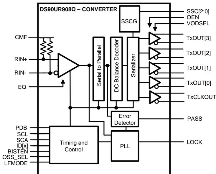
**Figure 1. FPD-Link II to FPD-Link Convertor**
