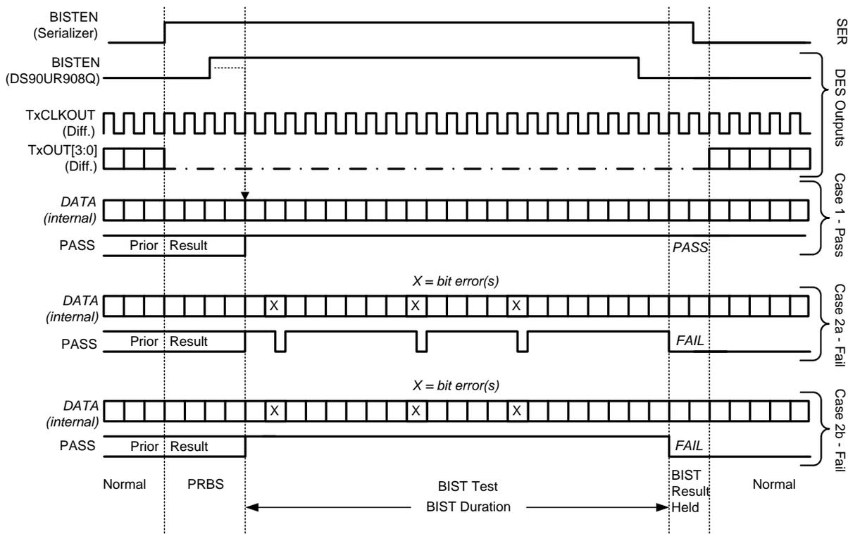
Figure 20. BIST Waveforms
