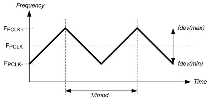
Figure 17. SSCG Waveform
