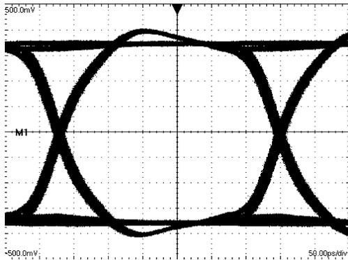
Figure 12. A 3.125 Gbps NRZ PRBS-7 Output Eye Diagram
