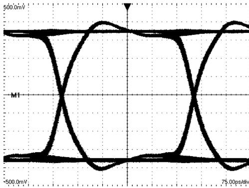
Figure 10. A 2.5 Gbps NRZ PRBS-7 Output Eye Diagram
