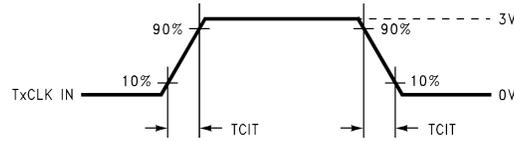
Figure 5. DS90CF383B (Transmitter) Input Clock Transition Time
