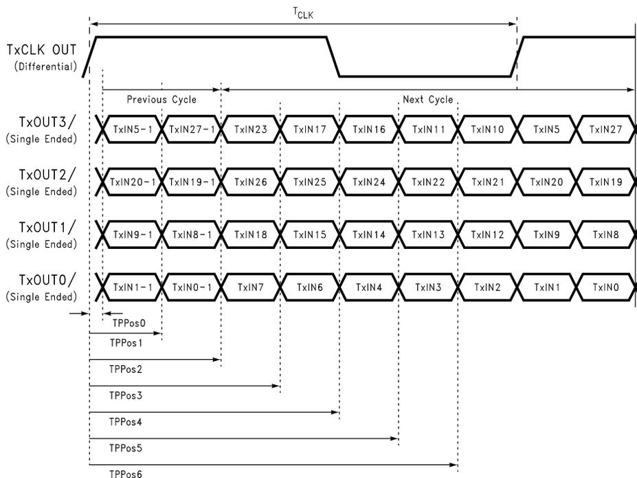
Figure 11. Transmitter LVDS Output Pulse Position Measurement
