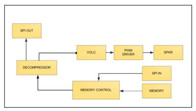
Figure 9-1 ISD2360 Signal Path
