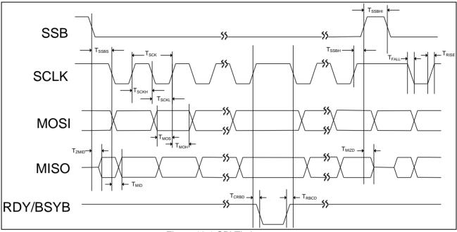
Figure 12-1 SPI Timing
