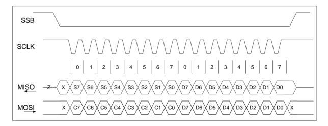
Figure 8-1 SPI Data Transaction.
