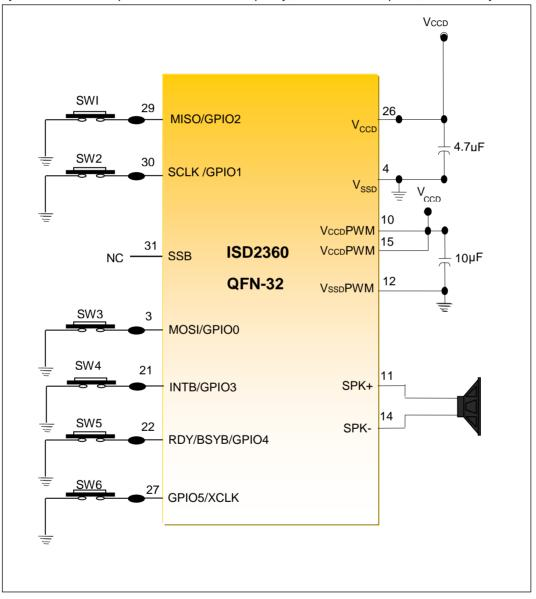
Figure 135-2 ISD2360 Application Diagram Stand-Alone Mode
