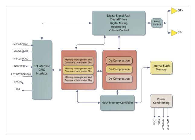
Figure 3-1 ISD2360 Block Diagram
