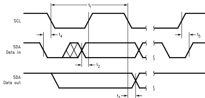
Figure 51. I<sup>2</sup>C Timing Diagram
