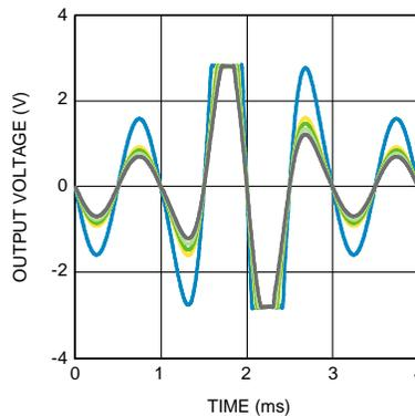
Figure 56. Clip Control Levels
