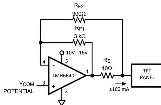
Figure 1. Typical Application as a TFT Panel  $V_{COM}$  Driver
