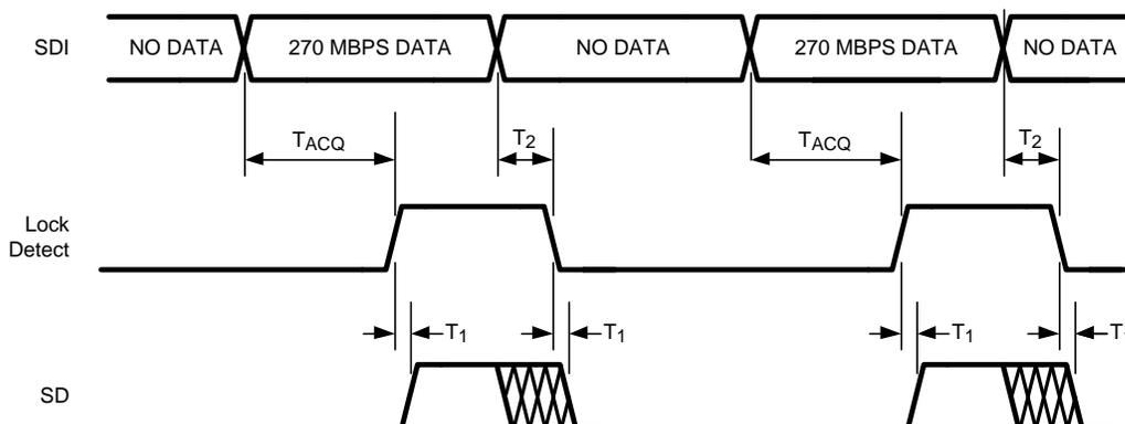
$T_{ACQ}$  = Acquisition Time, defined in the AC Electrical Characteristics Table
