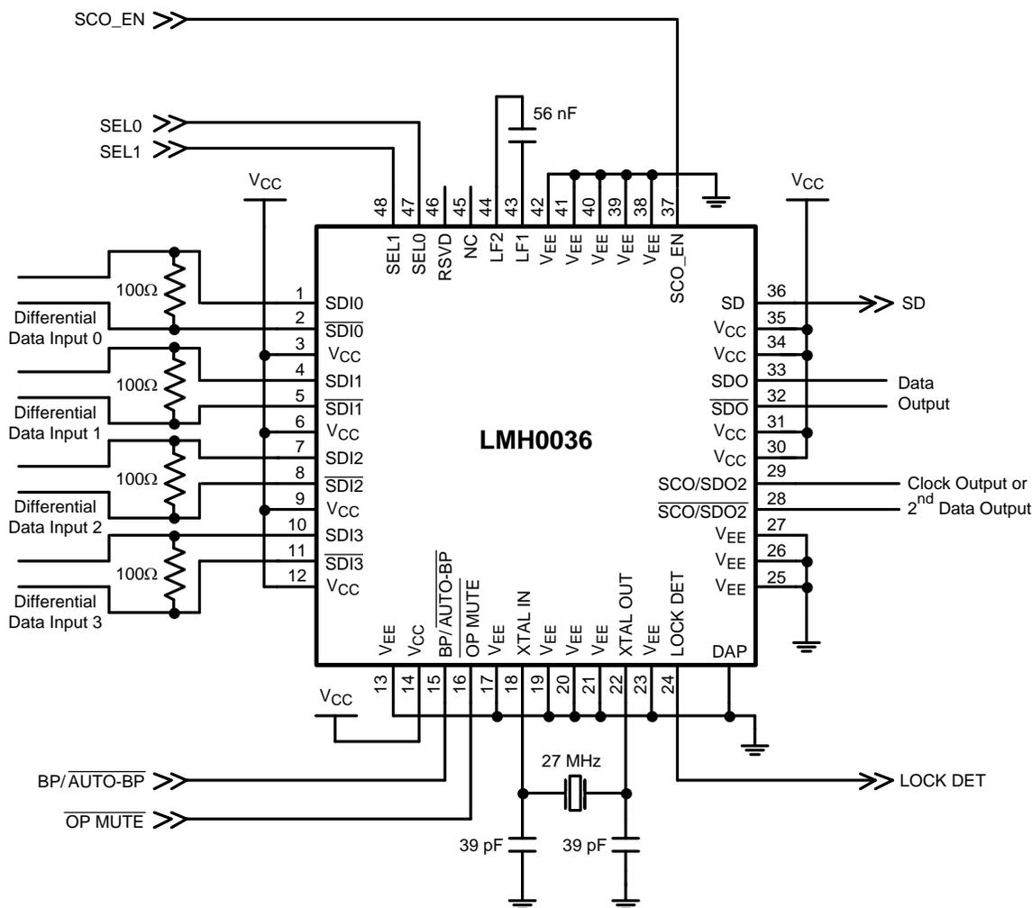
Figure 5. Application Circuit
