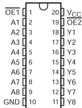
**Figure 5-1. D or PW Package (Top View)**
