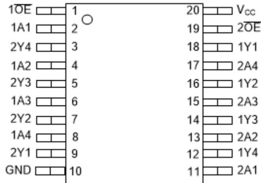
**Figure 5-1. DW or PW Package (Top View)**
