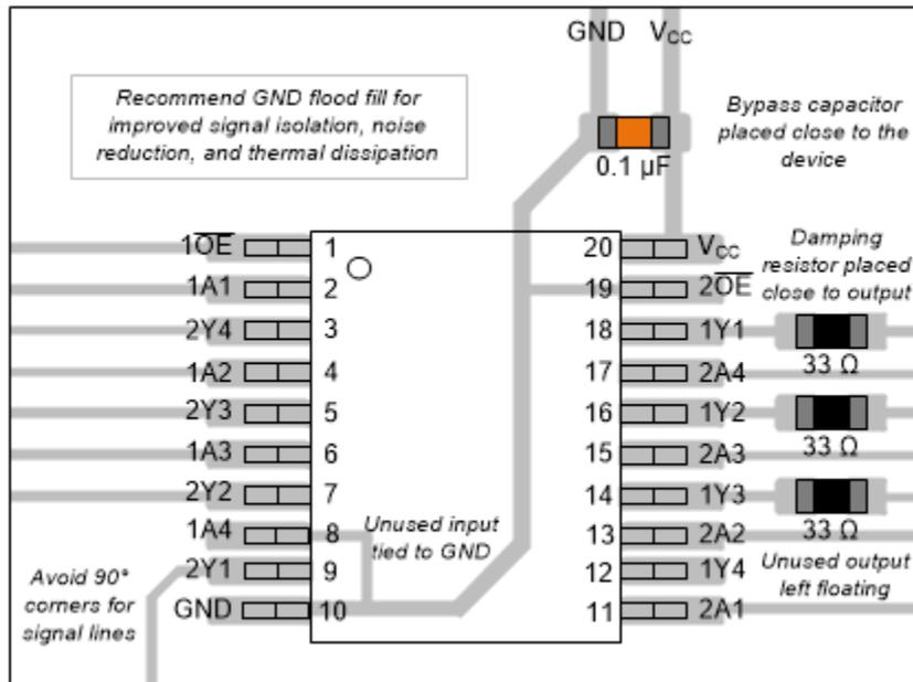
Figure 9-1. Layout Diagram
