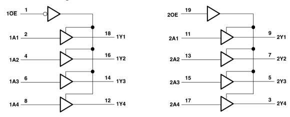
Figure 6-1. Logic Diagram (Positive Logic)
