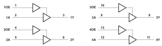
A. Pin numbers shown are for the D, DB, DGV, J, N, NS, PW, and W packages.
