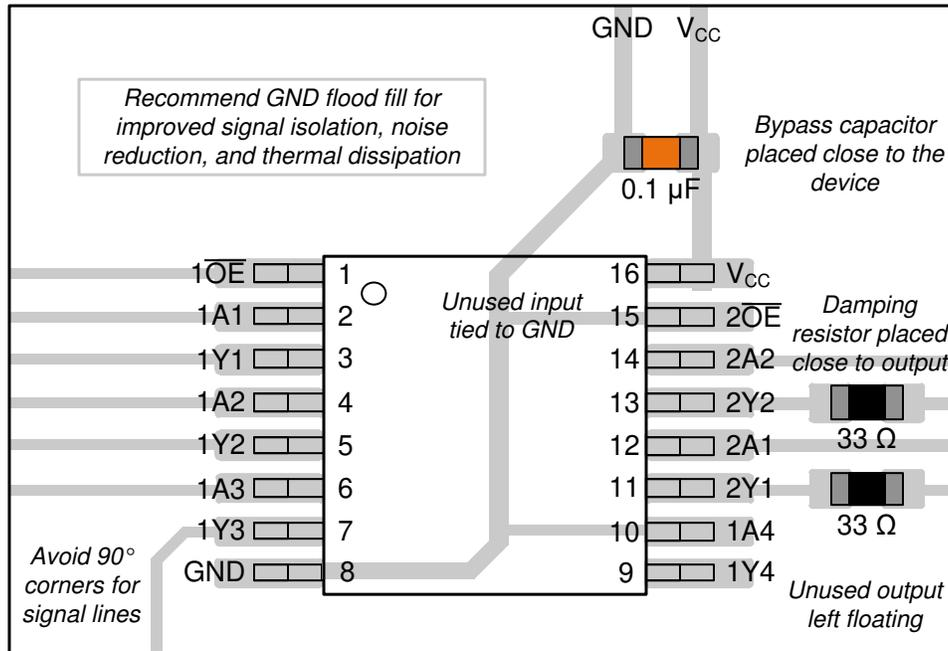
Figure 9-2. Example Layout for the SN74AHC367
