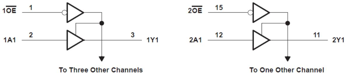
Figure 8-1. Logic Diagram (Positive Logic)
