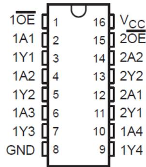
Figure 5-1. D, DB, DGV, N, or PW Package (Top View)
