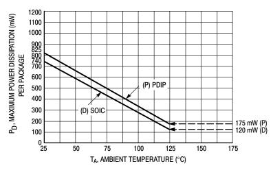
Figure 3. Ambient Temperature Power Derating
