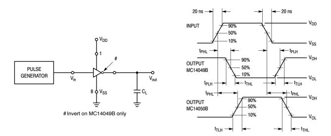
Figure 4. Switching Time Test Circuit and Waveforms
