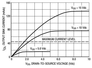
Figure 2. Typical Output Sink Characteristics
