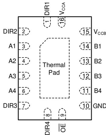
**Figure 4-5. BQB Package, 16-Pin WQFN, Transparent (Top View)**
