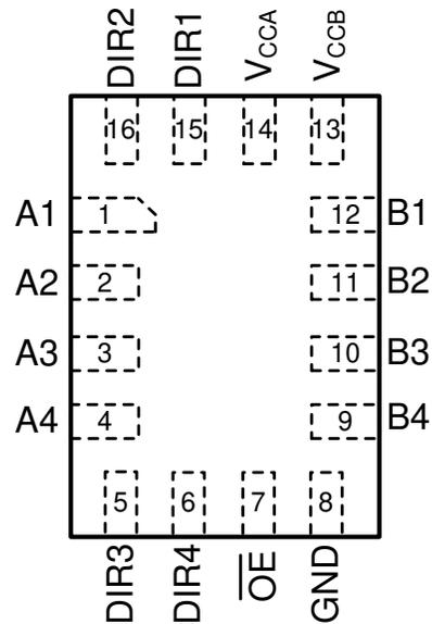
**Figure 4-4. RSV Package, 16-Pin UQFN (Top View)**
