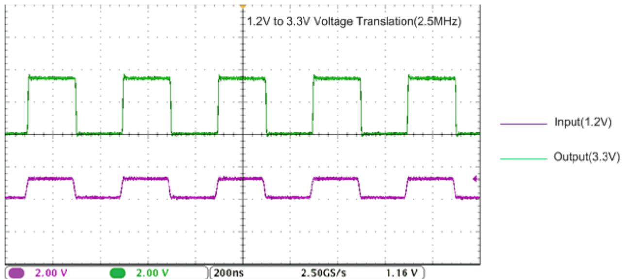
Figure 8-2. Translation Up (1.2 V to 3.3 V) at 2.5 MHz
