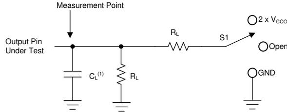
A.  $C_L$  includes probe and jig capacitance.
