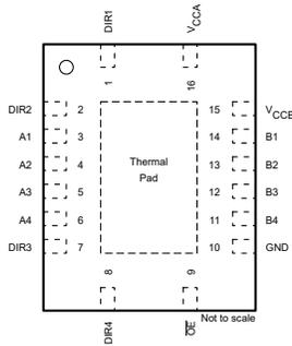
**Figure 4-3. RGY Package, 16-Pin VQFN (Top View)**
