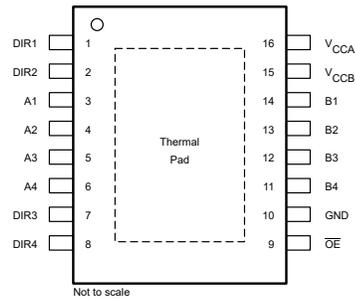
**Figure 4-2. DYY Package, 16-Pin SOT (Top View)**
