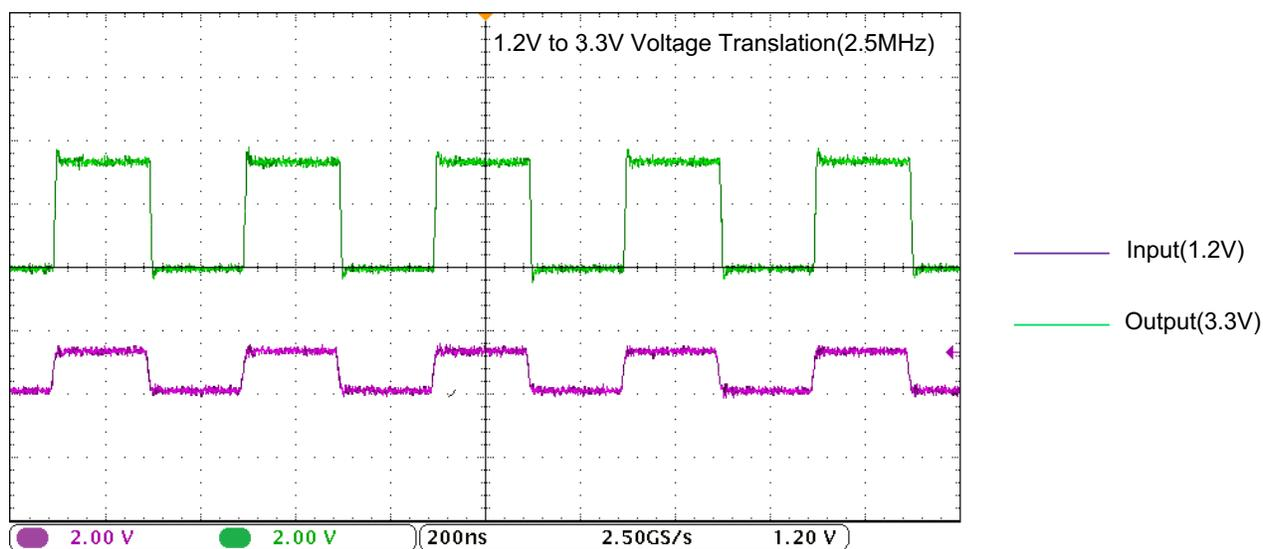
**Figure 8-2. Translation Up (1.2V to 3.3V) at 2.5MHz**
