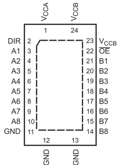
**Figure 4-2. RHL Package, 24-Pin VQFN (Top View)**
