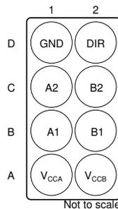
**Figure 5-2. YZP Package, 8-Pin DSGBA (Bottom View)**
