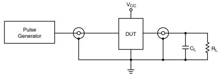
Figure 2. AC (Propagation Delay) Test Circuit
