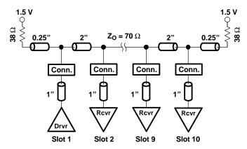
Figure 2. Medium-Drive Test Backplane
