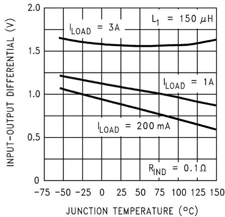
**Figure 6-3. Dropout Voltage**
