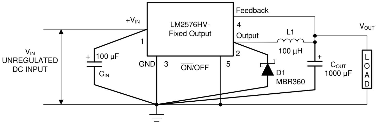
$C_{IN}$  — 100- $\mu$ F, 75-V, Aluminum Electrolytic  $C_{OUT}$  — 1000- $\mu$ F, 25-V, Aluminum Electrolytic  $D_1$  — Schottky, MBR360  $L_1$  — 100  $\mu$ H, Pulse Eng. PE-92108  $R_1$  — 2 k, 0.1%  $R_2$  — 6.12 k, 0.1%
