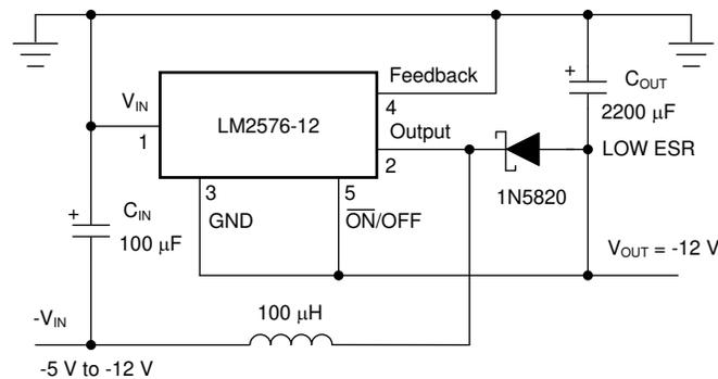
Typical Load Current 400 mA for  $V_{IN} = -5.2$  V 750 mA for  $V_{IN} = -7$  V Heat sink can be required.
