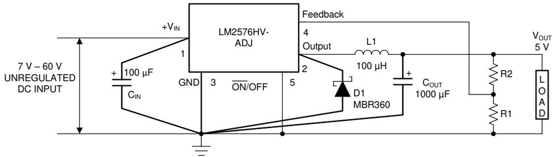
$$V_{OUT} = V_{REF} \left( 1 + \frac{R_2}{R_1} \right)$$
