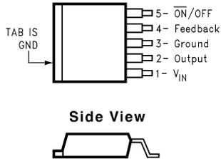
**Figure 5-2. KTT Package 5-PIN DDPAK/TO-263 Top View**
