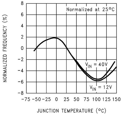
**Figure 6-7. Oscillator Frequency**
