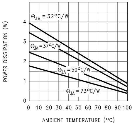
If the DDPAK/TO-263 package is used, the thermal resistance can be reduced by increasing the PCB copper area thermally connected to the package. Using 0.5 square inches of copper area,  $\theta_{JA}$  is 50°C/W, with 1 square inch of copper area,  $\theta_{JA}$  is 37°C/W, and with 1.6 or more square inches of copper area,  $\theta_{JA}$  is 32°C/W.
