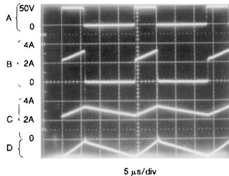
$V_{OUT} = 15\text{ V}$  A: Output Pin Voltage, 50 V/div B: Output Pin Current, 2 A/div C: Inductor Current, 2 A/div D: Output Ripple Voltage, 50 mV/div, AC-Coupled
