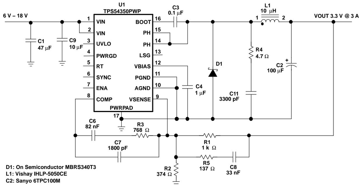
Figure 25. 3.3-V Power Supply With Schottky Diode
