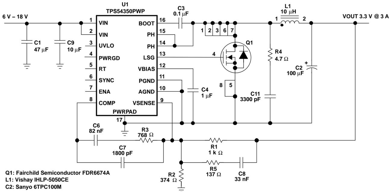
Figure 24. Application Circuit, 12 V to 3.3 V
